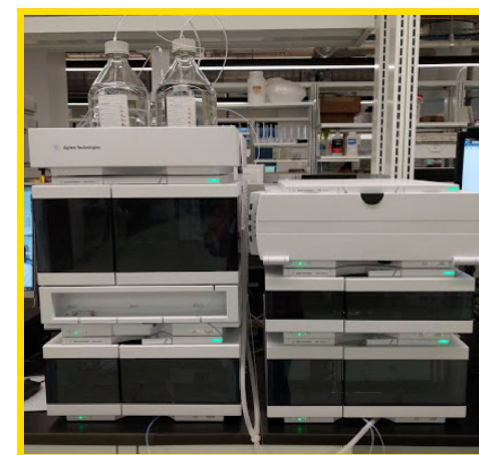
FIGURE 5: HIGH PERFORMANCE LIQUID CHROMATOGRAPHY IS USED TO SEPARATE AND QUANTIFY THE AMOUNT OF CRCs DRAWN INTO EACH FILTER.
