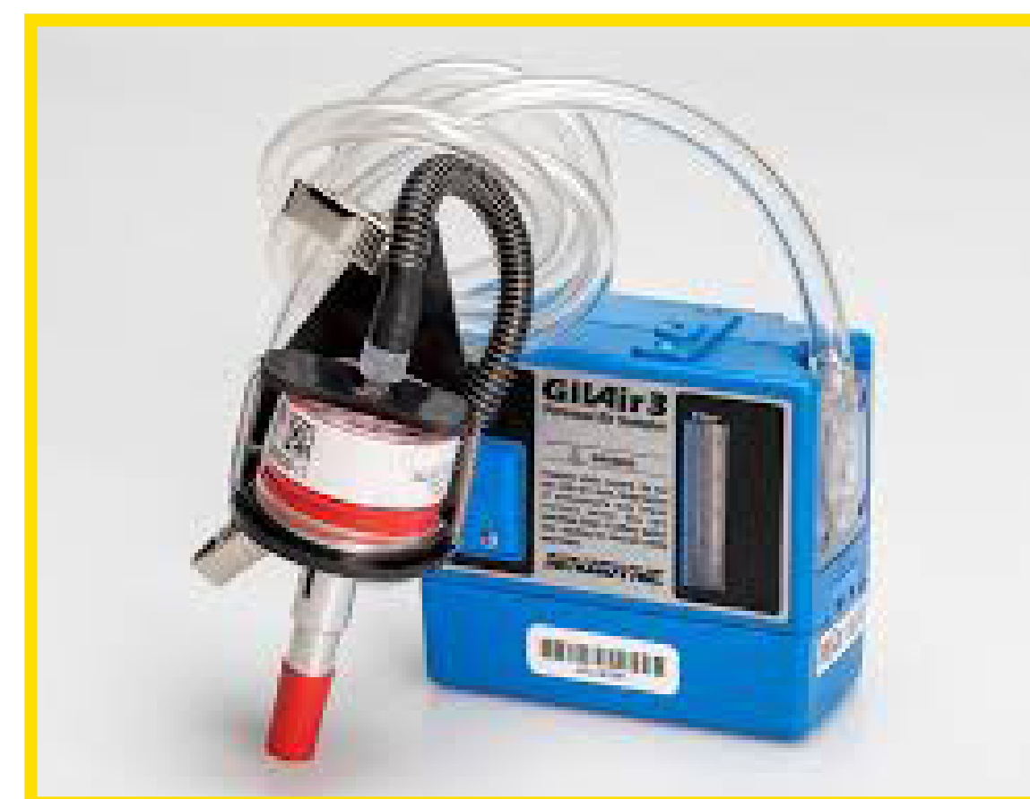
FIGURE 3 & 4: LAMPERD’S PEPPER SPRAY WILL BE DEPLOYED AND DUST SAMPLING PUMPS AND FILTERS WILL BE SET UP WITHIN THE PEPPER CLOUD RANGE. KNOWING THE VOLUME OF AIR THE PUMP WILL DRAW IN, THE AMOUNT OF CRCs IN THE AIR CAN BE CALCULATED.
